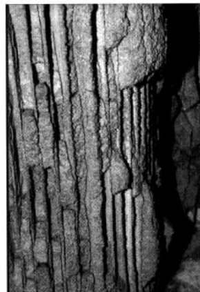
Fig. 18: Example of a very dirty pleated filter (spray granulation process). Severe decrease in the filter area on the product side, experiences considerable cleaning problems.
