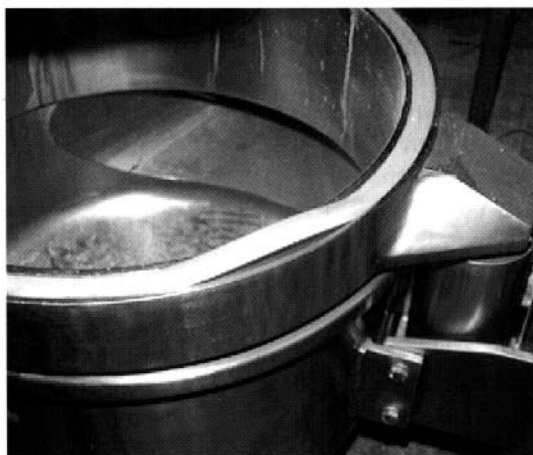
Fig. 2: A conventionally-designed flange. With this shape, either the product or the cleaning compound can infiltrate into the seal.
