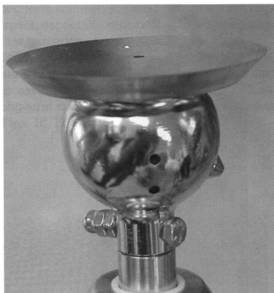
Fig. 22: Extendible cleaning nozzles, CIP-compatible design (Glatt, Binzen).
