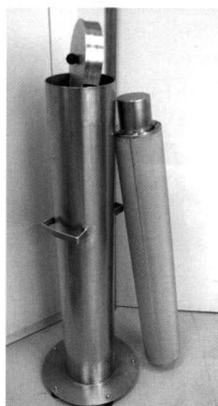
Fig. 21: Example of an immersion tank. With the use of a displacement body, the required solvent volume is reduced.
