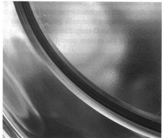
Fig. 11: Set-up showing the seal installed, CIP-compatible design (O-Plus™ System, Glatt, Binzen).
